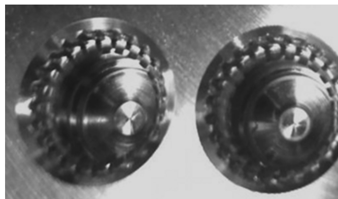
Figure 10. Holes after the broaching process [1].
