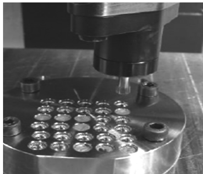
Figure 9. Experimental setup with special toolholder between tool and machine spindle [1].
