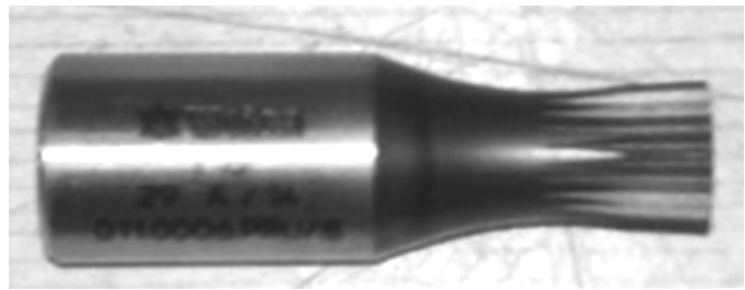
Figure 6. Typical shape of the used broach.
