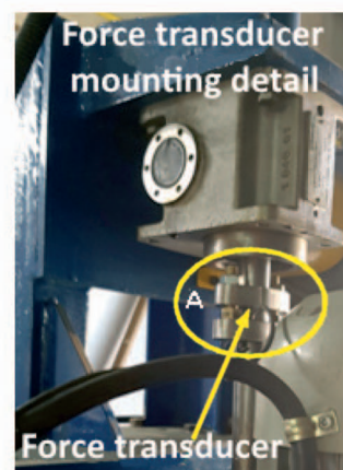
Figure 3. FSW machine interfaced with temperature and force monitoring systems.
