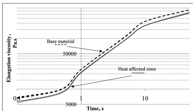
Figure 7. Recorded curve of the elongation viscosity.
