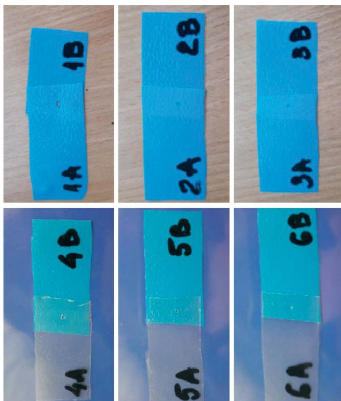
Figure 3. Welded specimens.
