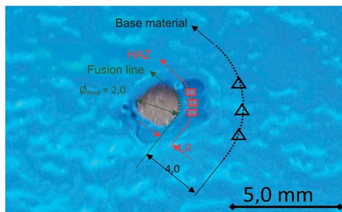
Figure 5. Locations to cut out samples for DSC.
