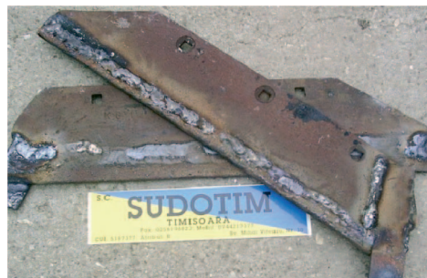
Figure 5. Plow equipped with self-sharpening modulated elements.
