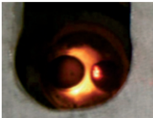
Figure 4. Snapshot during microwave heating of BaCO 3 composites materials.
