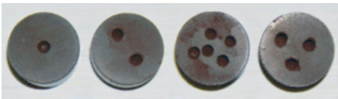
Figure 1. Composite with defects.
