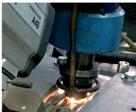
Figure 10. FSW-IG welding process sequence of TiGr2
