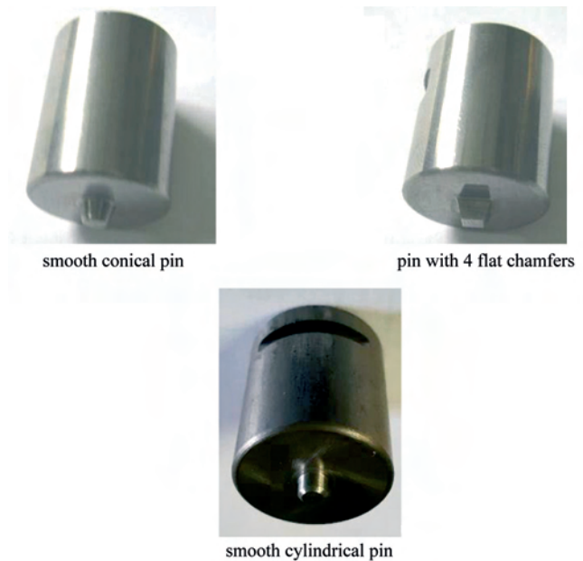
Figure 7. Welding tool geometries for FSW-IG processes
