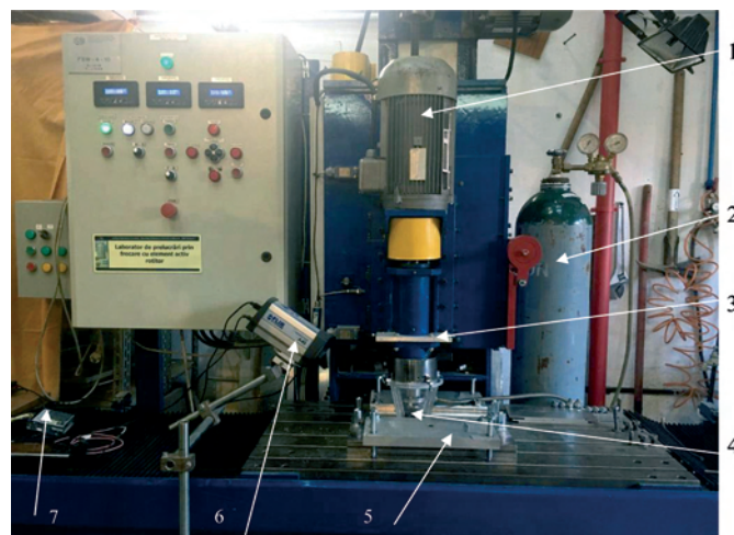
Figure 4. Variant 3 of shielding gas supply on the FSW machine
