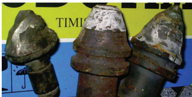
Figure 1. Effects of wear and blocking of knives after asphalt processing
