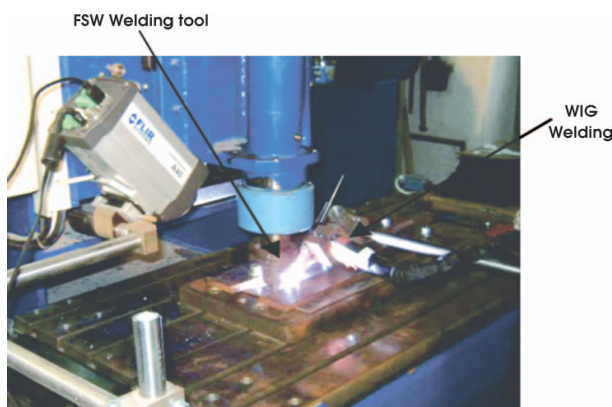
Figure 1. FSW-TIG Hybrid Welding Assembly
