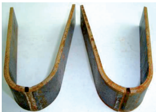
Figure 11. Samples welded with welding FSW-TIG steel S235JR+N.
