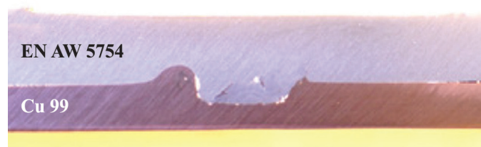
Figure 14. Macroscopic analyze of FSW weld EN AW 5754 - Cu 99.
