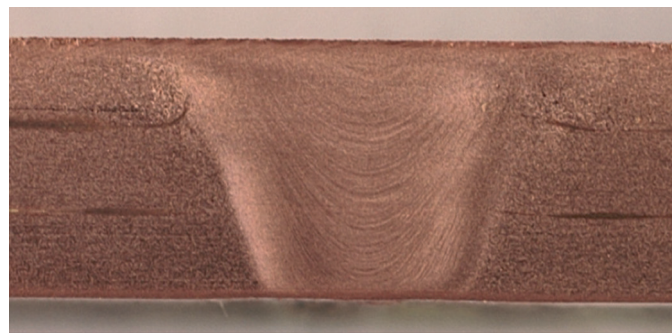
Figure 7. Friction stir lap welding of Cu 99 (2 mm/2 mm/2 mm).
