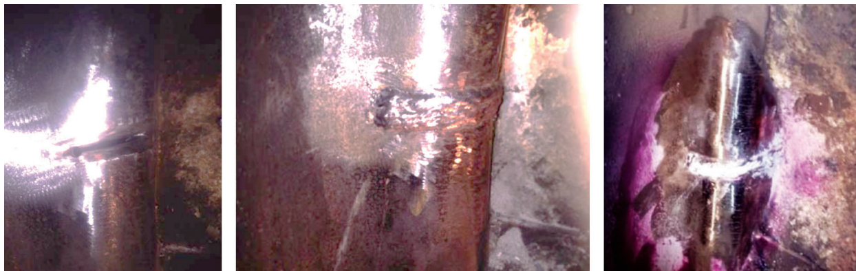
Figure 2. Cracks across the whole thickness of wave furnace tube.
