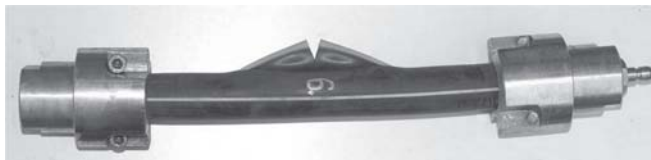
Figura 1. Rupere ductilă – Material de bază/ Figure 1. Ductile fracture – Base material
