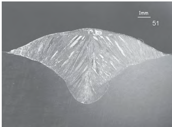
Parametri / Operational conditions ( v = 0.8 m/min, v_w = 14 m/min, P = 2 kW, I = 357 A, U = 29,5 V, foc.pos. = +10mm) Dimensiuni / Cord dimensions (L = 12,62mm, H = 1,84mm)
