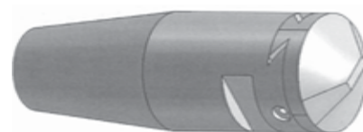
Figure 3. Electrode with prismatic working head
