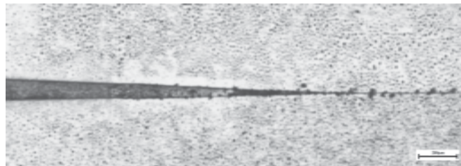
Figure 7. Microscopic image of the centre of brazed joint
