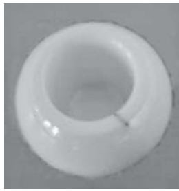
Figure 5. Ceramic head with crack
