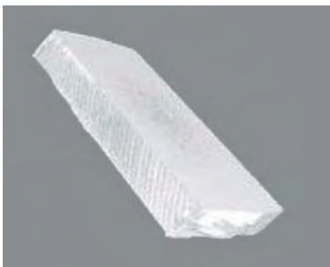
Figure 14. Absence of porosity in the FSW specimen
