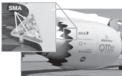
Figure 7. Commercial aircraft aero-engine showing adaptive serrated nozzle actuated by SMAs (on top)
