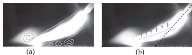
Figure 15. Fluid-dynamic effect (a) and thermal effect (b) on a welding arc trajectory
