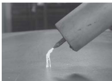
Figure 12. Very low current arc obtained through a high-frequency igniter and low Argon flow showing the change in plasma orientation
