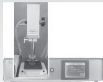
Cavitation equipment, 500 W / 20 kHz
