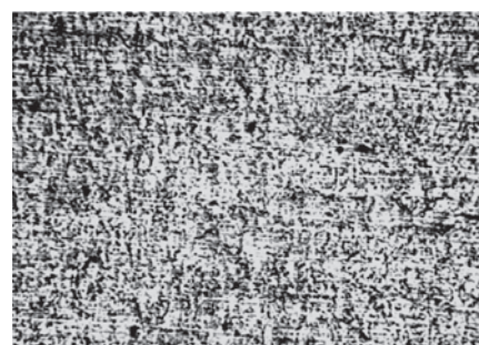
Figure 5. Base metal microstructure, 100x.
