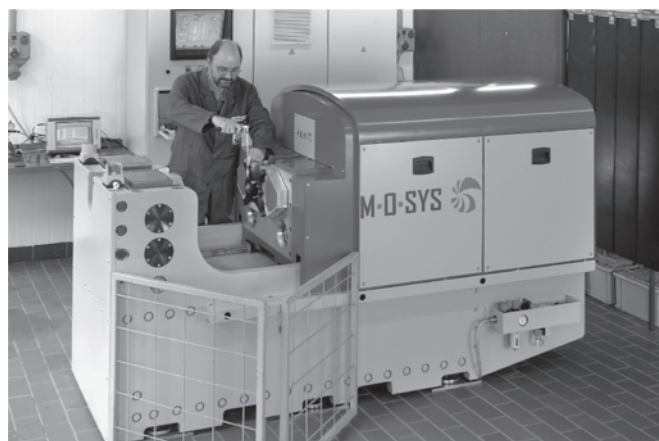
Figure 3. Multi-orbital friction welder of the MOSYS RSM100 type with a pressing-on force up to 100 kN.
