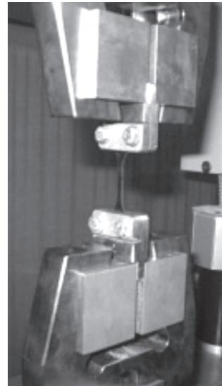
Figure 5. Fixing system of specimen
