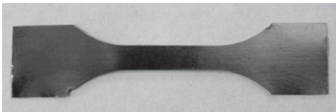
Figure 4. The specimen with calibrated portion used for tensile test
