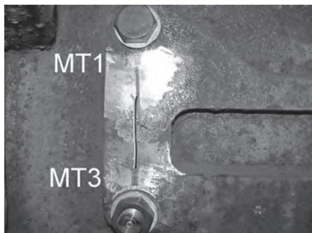
Figure 8. points where measuring tapes are put.
