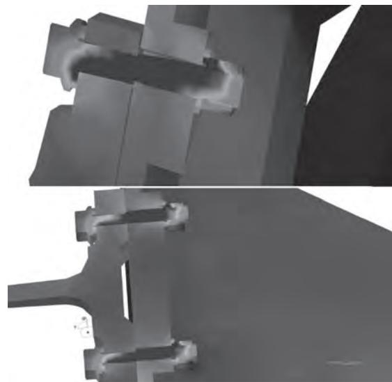
Figure 11. Bolts connections with the bus chassis turntable in unmodified condition where uneven load in the screws stem is visible.
