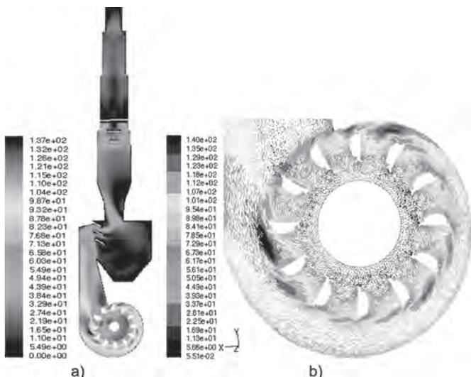
Figure 6. Field of absolute vectors' velocity mixture in a vertical plane passing through the axis of rotation (a) in the mill around the striking plates (b).
