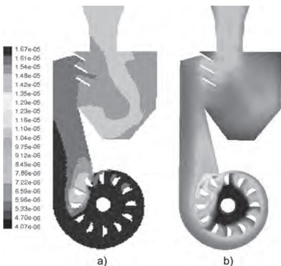
Figure 7. Volume concentration of sand (a) and turbulence of mixture (b).
