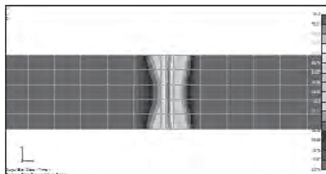
Figure 3. The detail stress distribution in welding area of specimen.
