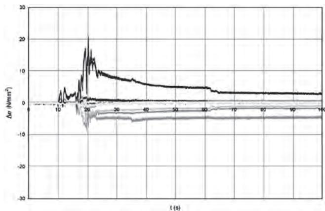
Figure 10. Stress state during crossing of the left bus wheel through barriers of 150mm.
