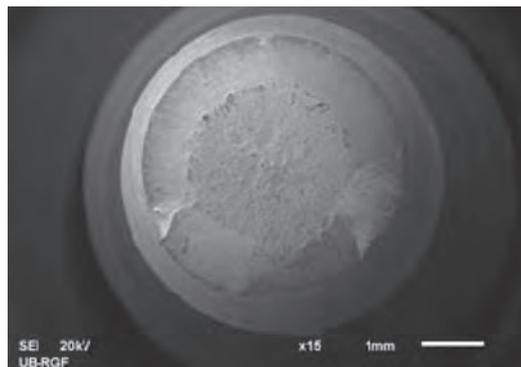
Figure 14. Macrographic view of the broken bolt, where can be observed crack initialization zone, which characterizes predominantly ductile fracture
