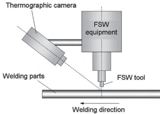
Figure 12. Scheme of positioning for thermographic camera on FSW machine.
