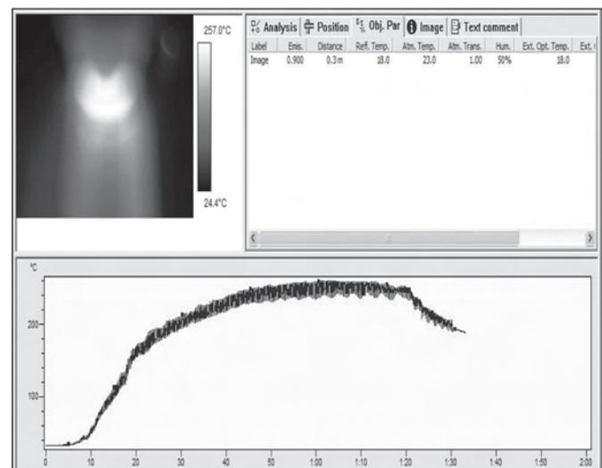
Figure 9. Temperature evolution during FSW deposition process, using tools having  $\Phi 20$ mm, made from EN AW 5086 ( $v=200$  mm/min).
