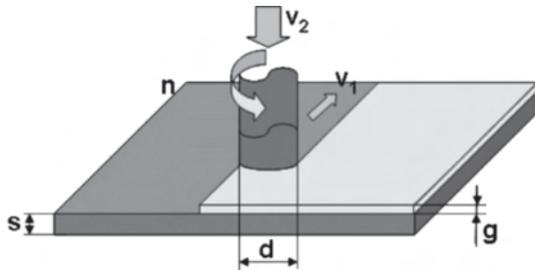
Figure 5. Scheme of deposition procedures.
