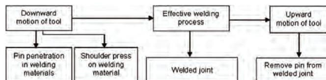
Figure 20. Sequences and stages of FSW process.
