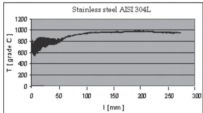
Figure 15. Evolution of temperature - AISI 304L, monitoring by infrared thermographic camera [5].
