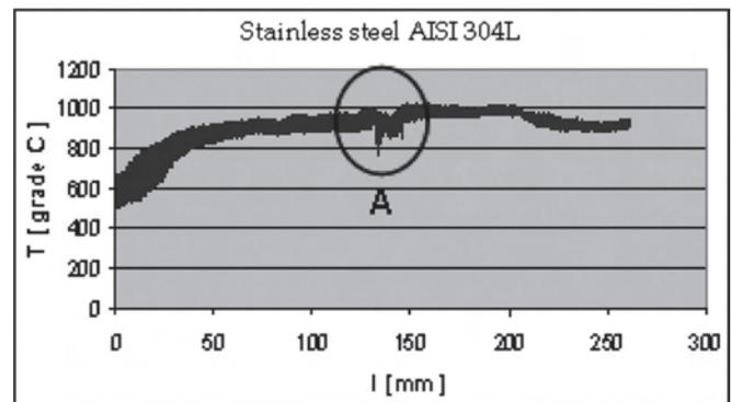
Figure 16. Detection of defect by thermography [5].
