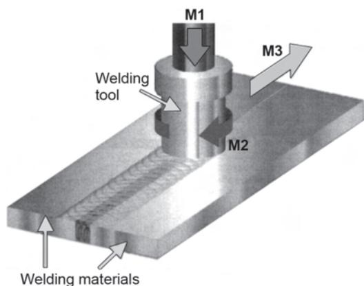
Figure 18. Friction Stir Welding process.
