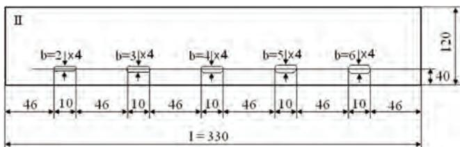
Figure 13. Sketch of samples with simulated defects [6].
