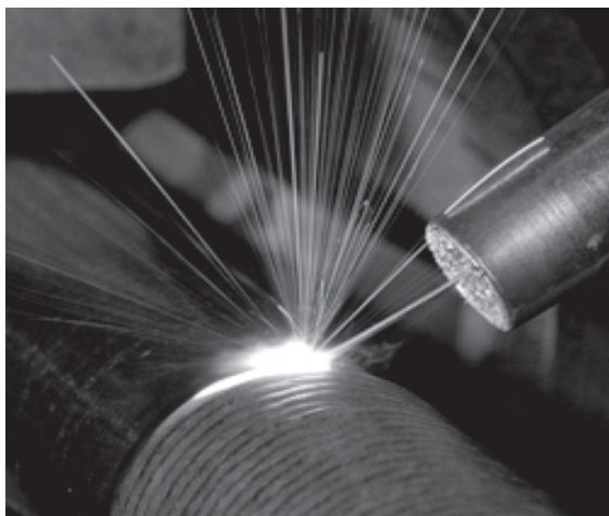
Figure 3. Hot-wire laser cladding [3] (laser head out of the frame).
