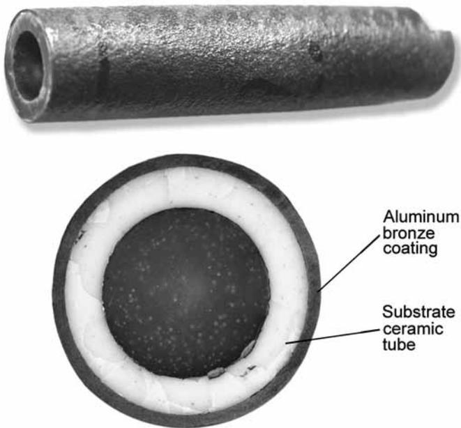
Figure 6. Macroscopic aspect of aluminum bronze coatings on ceramic tube.
