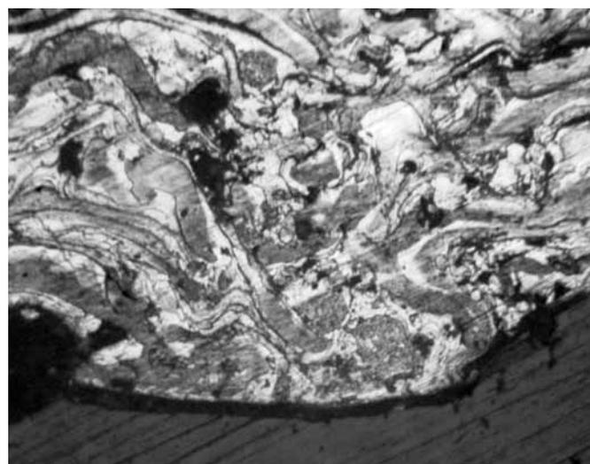
Figure 5. Microscopic structure of the depositions
