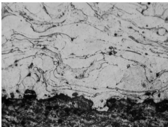
Figure 3. The microstructure of the deposited layers.
