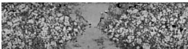
Figure 2. Macroscopic view (filler material: AlMg4.5Zr).
