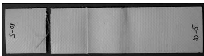
Figure 3.4. Rupture in base material, outside of the welded region, as result of tensile testing (welding condition 10).
