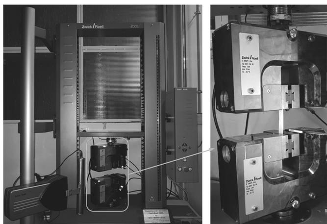
Figure 2. Equipment Zwick/Roell Z005 – 5kN / Detail on the active jaws level.
