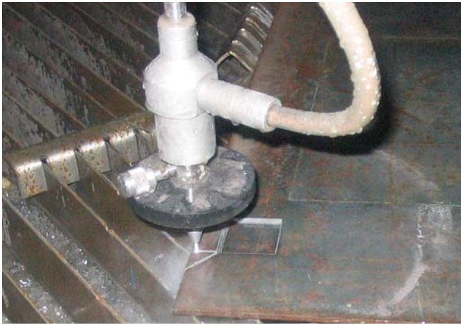
Figure 2. Abrasive water-jet cutting process on a 10 mm steel plate.
