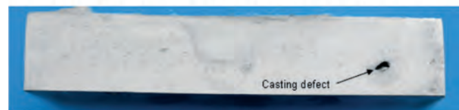
Exp. 2.2 - conical pin with 4 flat chamfers, v = 200 mm/min
