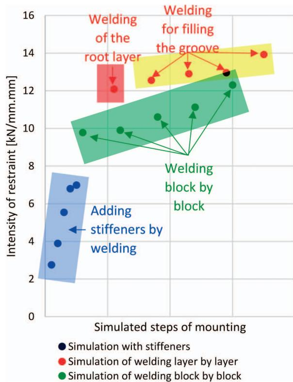
Figure 5. Intensity of restraint as calculated by FEM simulation.
