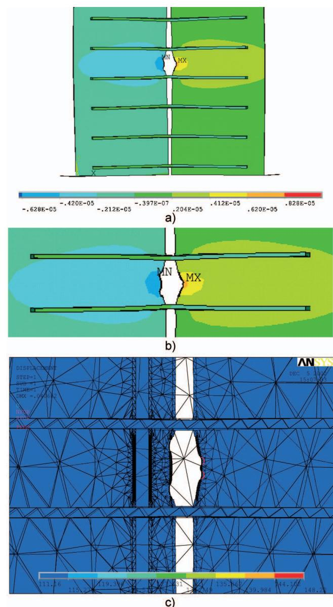
Fig. 4 Geometrical model connected with compression bars (a.) and the displacement error given by the compression bars (b.)
