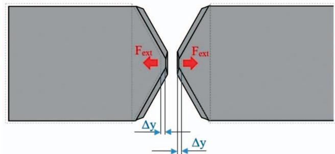
Figure 1. Geometrical elements used to calculate the intensity of restraint.
