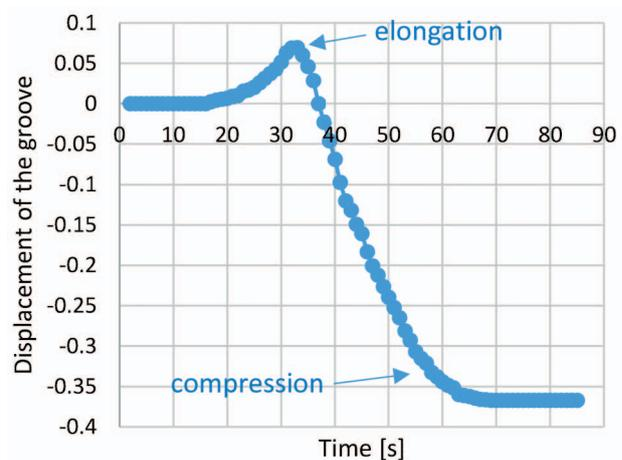
Figure 7. Deformation by welding sequence.
