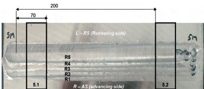
Figure 4. Appearance on the surface of the processed FSP material
