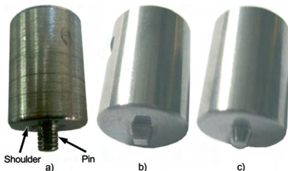
Figure 2. Processing tools used in the experimental program: a) Threaded cylindrical pin tool; b) Conical pin tool with 4 flat bevels; c) Smooth conical pin
