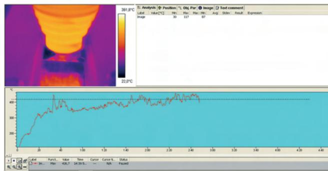
c) R3 - Exp. 3 ( $T_{R3 \text{ max}} \sim 455^{\circ}\text{C}$ ;  $T_{R3 \text{ med}} \sim 420^{\circ}\text{C}$ )
