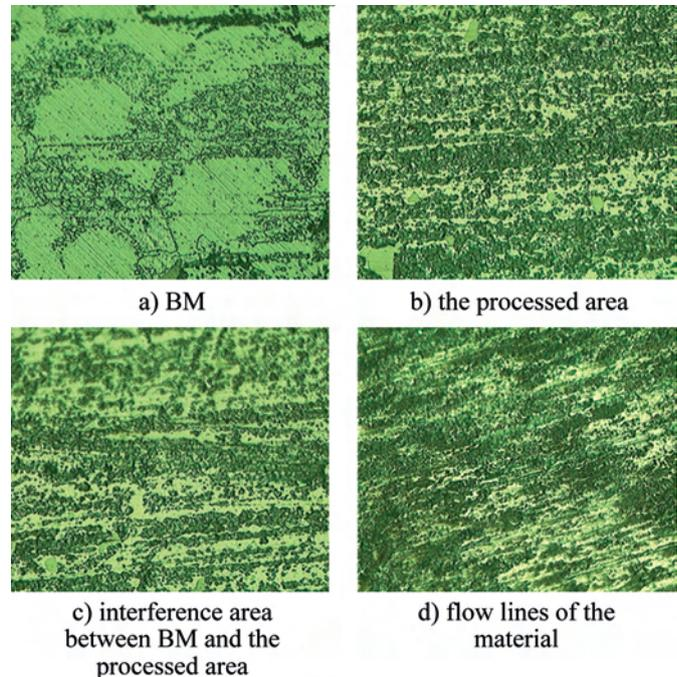
Figure 6. Microstructural analysis for the base material and processed material
