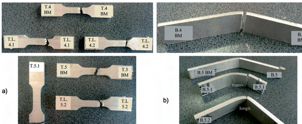
Figure 8. Appearance of specimens taken from the processed material and BM (Exp.1, 2) tested at: a) tensile tests (T); b) bending tests (B)
