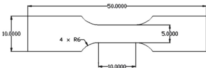
Figure 7. Sketch of small dimensional specimen for tensile test
