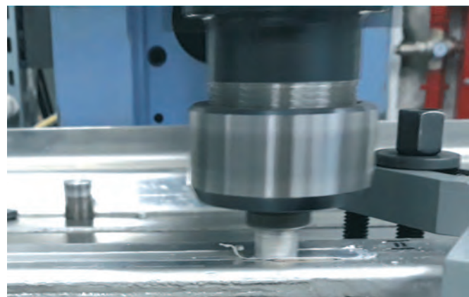
Figure 6. Execution by FSP of the pass 2, to improve the initial FSW welding, at the joint with mark II.
