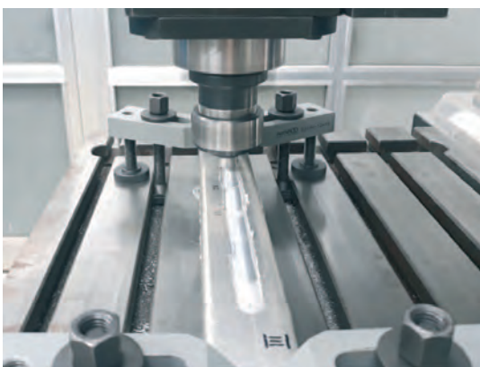
Figure 9. Execution of the FSP 9.4 pass, over the FSP 9.3 run, of the mark III joint.
