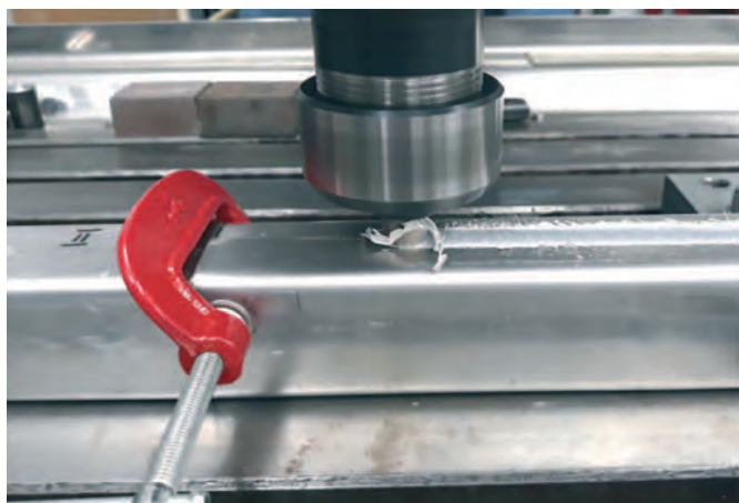
Figure 4. Execution by FSW of the welding (pass) 1.1 of the mark I joint.
