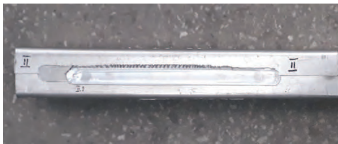
Figure 12. The 45 mm x 45 mm square tube (test piece) welded by FSW and corrected by FSP, on the generator line, made of aluminum alloy sheets with steel core, in the final stage.
