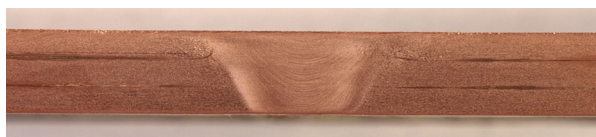
Fig. 9. FSW overlap welding - Cu 99 [19]
