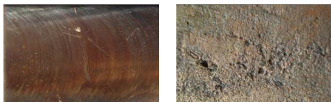
Fig. 15. Comparison - casted and FSP processed bronze FSP [19]
